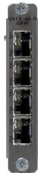
UVTX/UVRX H264 SFP Rear Panel (Optical)
